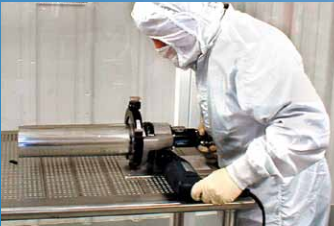
Solution Profile: Stainless thin wall tubing being cut in a cleanroom for a high purity tubing system. The Model 304 produces a perfectly square, burr free end ideal for orbital welding procedures.
