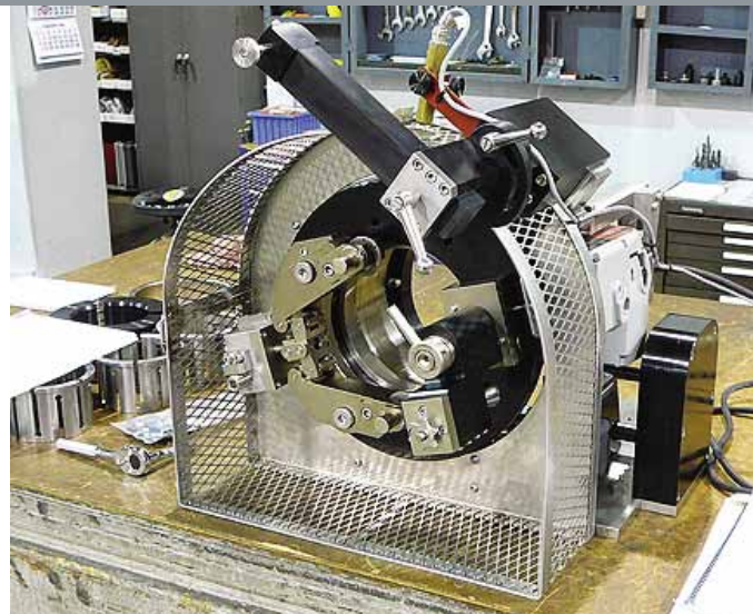
Solution Profile: This 576 AC SeverMaster® was designed for use in a glove box. Configured with roller cutters, it performs remote chipless cannister opening. Other unique features include a pivoting base stand, laser pointer for cut location reference and a burnishing module to push the burr out of the way to allow removal of the inner can.
